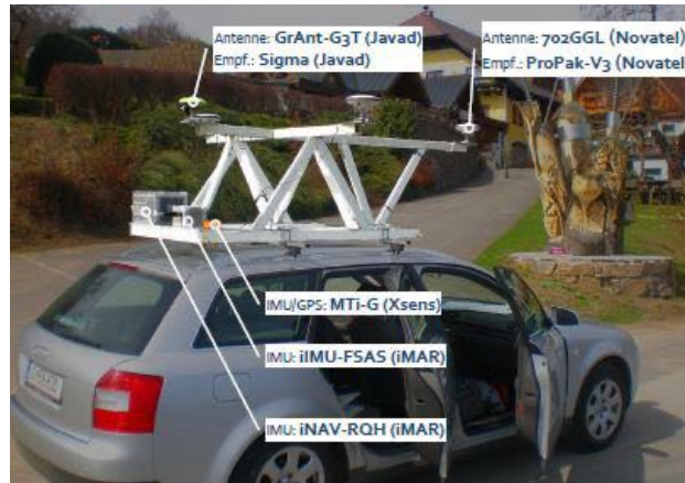
Figure 2: GNSS and IMU sensors mounted on the private car's roof [laengauer,2010]
