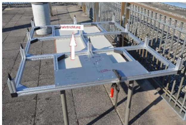
Figure 3: tailored calibrated platform applied for the sensor fusion [Wieser, 2019]
